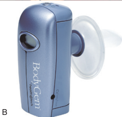
FIGURE 6-2 (A) MedGem and (B) BodyGem devices, which are used to determine the resting metabolic rate. (Courtesy Microlife USA, Dunedin, FL.)
