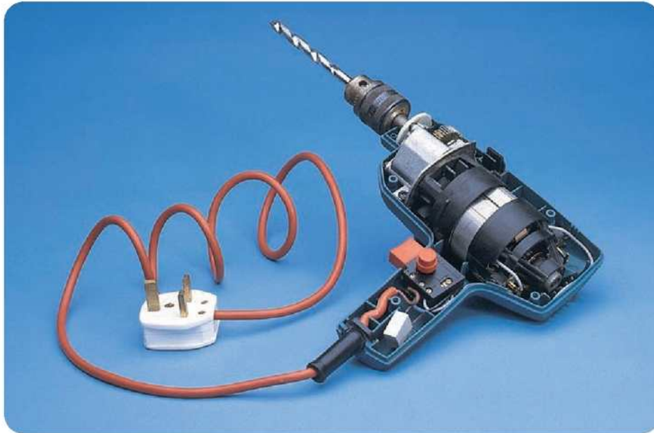
◀ In this electric drill, the motor is in the centre. Note the commutator segments at the right hand end, and the electromagnet.
