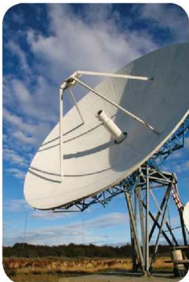
▲ This dish receives microwaves from a satellite.
