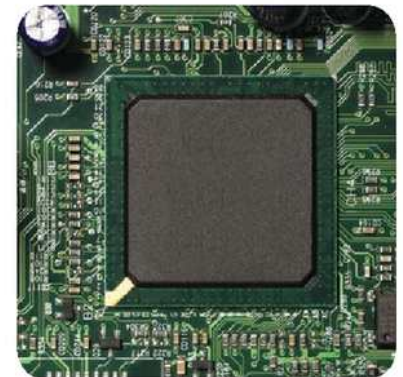
▲ A microprocessor like this contains over 100 million logic gates.
