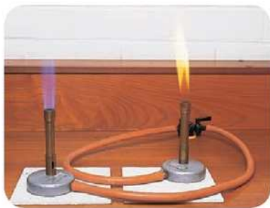
▲ A yellow bunsen flame is easier to see than a blue one.
