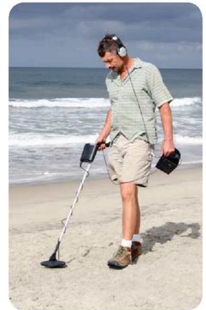
▲ A metal detector creates eddy currents in metal objects and then detects the magnetic fields produced.
