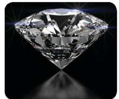
▲ When a diamond is cut, the facets (faces) are angled so that they produce total internal reflection. Reflected light gives the diamond its 'sparkle'.
