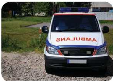
▲ The word on this vehicle is laterally inverted so that it reads correctly when seen in a driving mirror.
