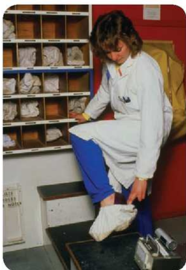
▲ This nuclear laboratory worker is about to use a GM tube and ratemeter to check for any traces of radioactive dust on her clothing
